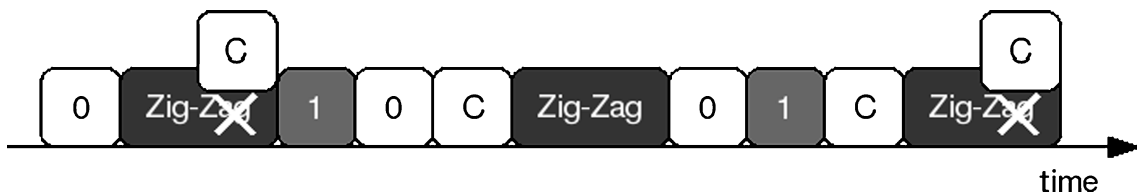
Fig. 4 A timeline of events in slotted Aloha. Two ZIGZAG frames are ruined by new arrivals on the second slot
